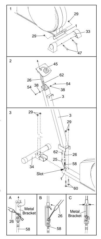
While a second person holds the Console (6) near the Console Bracket (45), connect the Extension Wire (62) to the console wire. Make sure the slack Resistance Cable (26) is pulled out of the Upright (3).
